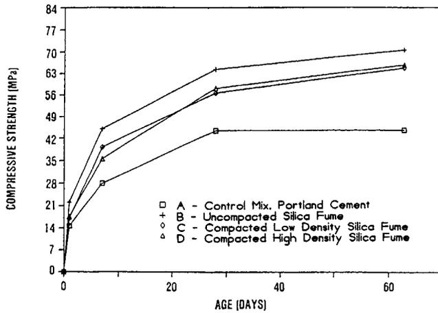
Fig. 1 — Compressive strength of wet-mix shotcrete.
