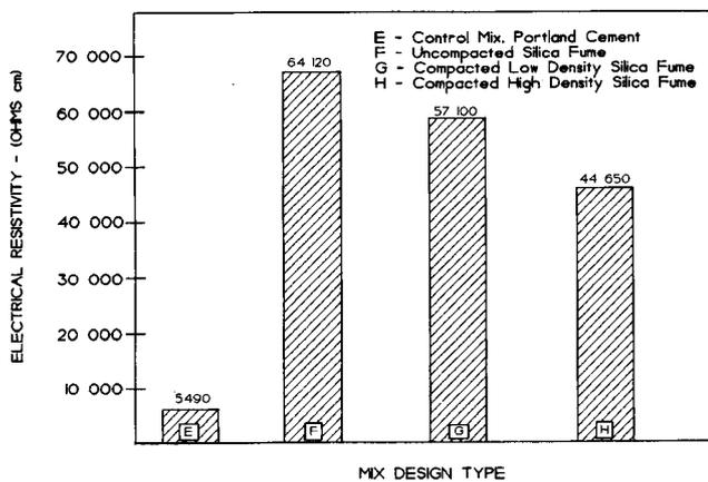
Fig. 6 — Electrical resistivity of dry-mix shotcrete.
