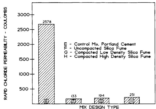
Fig. 4 — Rapid chloride permeability of dry-mix shotcrete.
