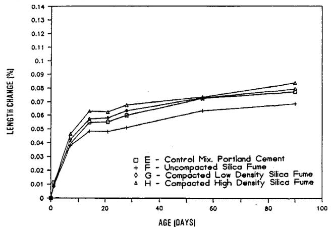
Fig. 8 — Drying shrinkage of dry-mix shotcrete.
