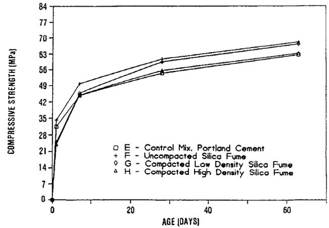
Fig. 2 — Compressive strength of dry-mix shotcrete.
