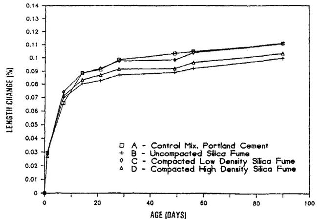
Fig. 7 — Drying shrinkage of wet-mix shotcrete.
