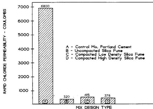
Fig. 3 — Rapid chloride permeability of wet-mix shotcrete.
