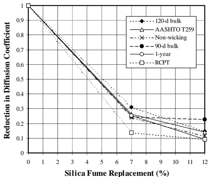
*Figure 7 - Relative reduction in diffusion coefficients with silica fume ( $W/CM = 0.35$ )*
